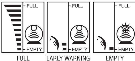
DIAGRAM 3 - Continuous display on small LCD Panel of Receiver 10 bar graph level display
